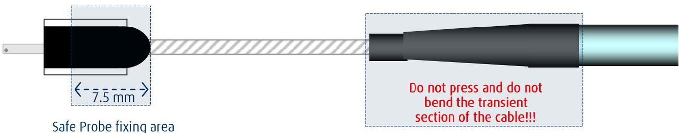
Figure 3. Safe fixing area of the E Probe head
