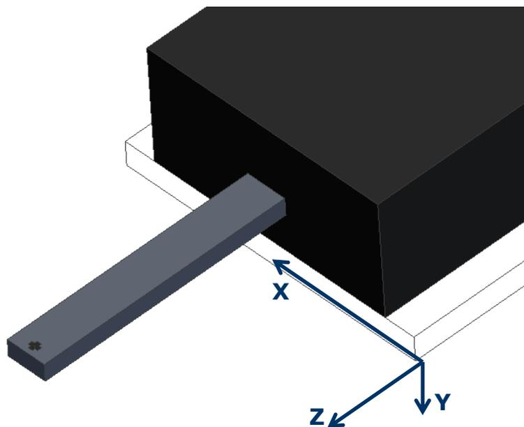
Figure 4: The reference Cartesian coordinate system of E probe
