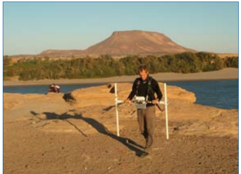
Prize winner: The Bartington Grad601 Gradiometer System pictured hard at work in Sai Island, Sudan
