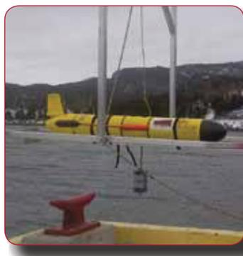
Underwater gliders used for environmental monitoring can navigate beneath the polar icecap with the help of Bartington Instruments' Mag648 sensor.
