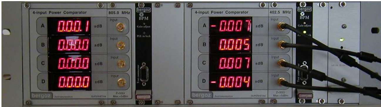
Shown on picture: Two 4-input RF Power Comparator in one chassis
